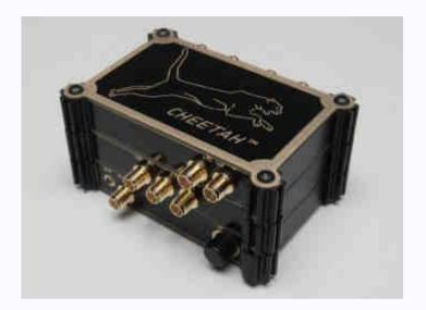
For frequencies above 30 MHz, the receiver is based on a double-conversion process, where the incoming frequency is down-converted to the output frequency 70 MHz, which is provided as a filtered output ready to be digitized. The IF paths are switchable by an internal relay in order to minimize images and spurious mixing products. Filters are specially selected to ensure flat phase response and a digitally controlled attenuator is employed in the front-end.
